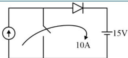
Energy loss  $10 \times 15 \times T_{OFF}$
