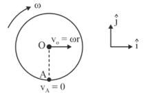
Since the disc is rolling without slipping hence velocity of point A;
