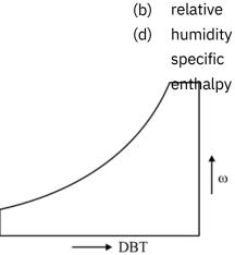
In psychometric chart x-axis represents dry bulb temperature and y-axis represents specific humidity.
