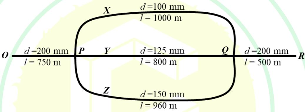
Diameter (*d*) and length (*l*) of each pipe are as presented in figure and all pipes are of same material having friction factor (*f*) of 0.02. Assume acceleration due to gravity (*g*) as 10.0 m/s<sup>2</sup>. If the head difference between *P* and *Q* is 10 m, then the head loss between *Q* and *R* is \_\_\_\_\_ m. (rounded off to two decimal places)
