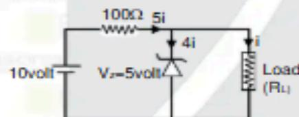
We have to assume that the zener breakdown is occurring. So the voltage across the zener diode is 5 volt. So the voltage across the series resistance will be
