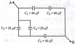
If C<sub>1</sub>, C<sub>2</sub>, C<sub>3</sub>, C<sub>4</sub>, C<sub>5</sub> five capacitors are connected in an electrical circuit as shown in figure, then calculate the equivalent capacitance of this mesh (network) between point A & point B.
