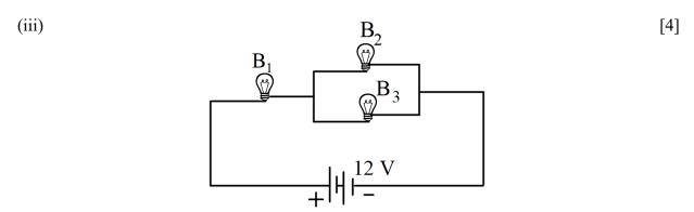
Three identical bulbs **B**<sub>1</sub>, **B**<sub>2</sub>, and **B**<sub>3</sub> each of power rating 18 W, 12 V are connected to a battery of 12 V.
