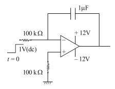
With respect to the figure above, the output voltage after 1 sec of the application of input voltage is
