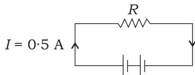
In the circuit shown above, each cell has an e.m.f. 2 V and an internal resistance of  $1 \Omega$ . The current flowing through the circuit is  $0.5$  A. The resistance of the resistor  $R$  is
