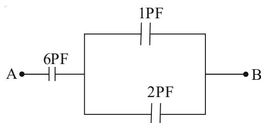
Determine the equivalent capacitance between the points A and B in the adjoining figure.
