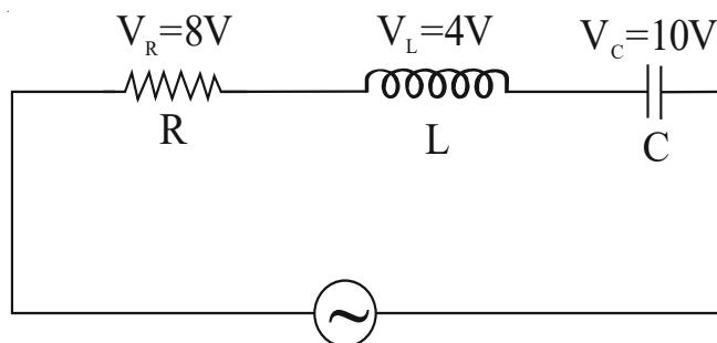
The value of alternating voltage in the following circuit is -
