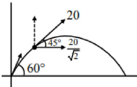
**Step 1:** Write horizontal component of velocity.
