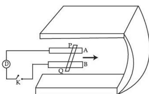
Suppose K is open and the rod is moved with a speed of  $12$  cms $^{-1}$  in the direction. The magnitude of the induced emf will be :
