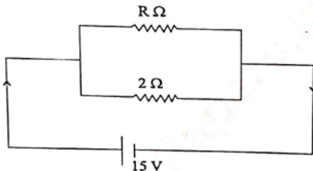
For the given following circuit diagram, the dissipated of electrical power  $150\ \text{W}$ , then find value of Resistance  $R = \text{_____}$ .
